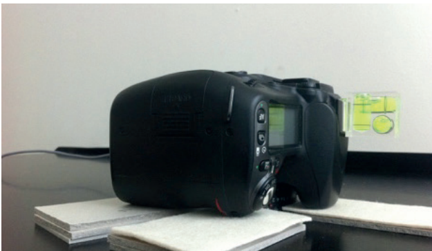
Figure 2 | The camera is levelled provisionally using pieces of cardboard and a bubble level with a hot shoe. On the inside you see the camera lens protruding through the ceiling of the box, fitted with a filter holder that contains a Kodak Wratten 2E filter.
